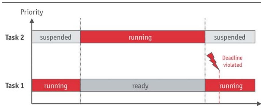
Figure 3. Deadline monitoring to detect deadline violations. The error source of Task 2 is not found in Task 1.
